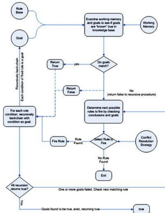
Gambar 1. Algoritma Metode *Backward Chaining*
